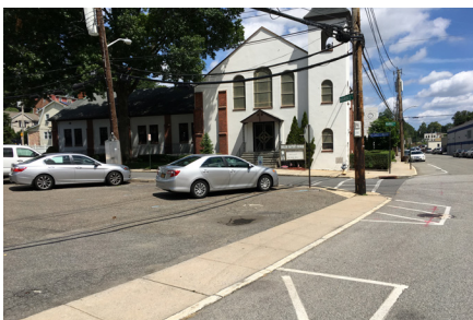
Poor definition between sidewalk and parking area
