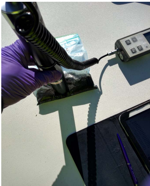
Sample Scanned Using 1x1 NaI Probe
