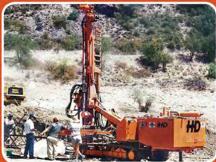
Cyprus - Soil Investigation Core Drilling Zypern - Bodenuntersuchung Kernbohrung
